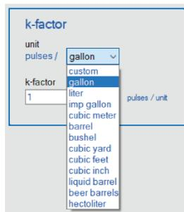
Select the units for the K-factor. Enter the number of pulses per unit. A value of 0.000001 to 9999999 can be entered.
