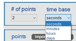
Select the number of scaling points. Up to 32 points can be selected. Select a unit of time in seconds, minutes, hours, or day in the time base menu.
