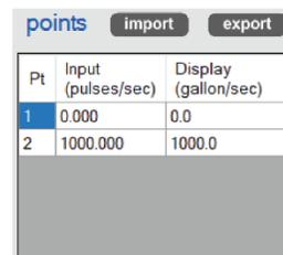
The scaling points can be entered directly into the software or imported from a .csv file. They can also be exported to a .csv file. This area also shows the input and display value for each point.
