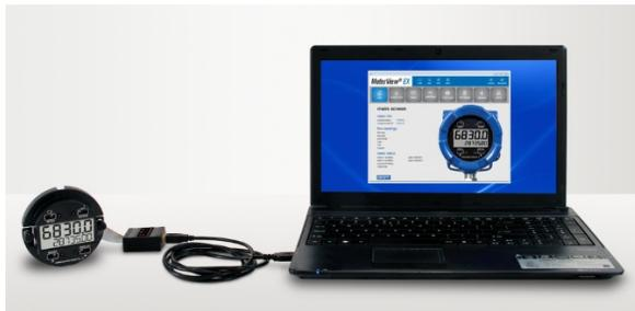
Free, PC-based, MeterView EX software that connects to the meter with the PDA8068 USB adapter is available for programming and setup of the flow rate/totalizers. This software greatly simplifies the programming process and allows the user to save configuration files for later use. The rate/totalizer will also be powered by the USB connection, so no additional power is needed during programming.
