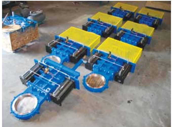
18" Bonnetless Knife Gates, 150 psi, 316 SS Trim, Expanded Metal Safety Guard, Hazardous Waste Disposal, Ohio
