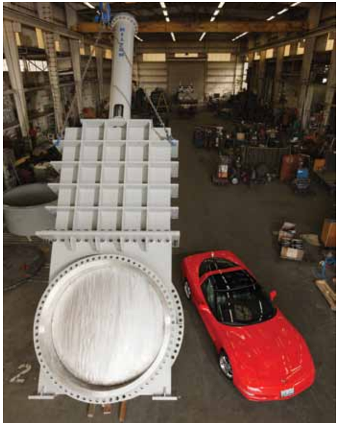
90" Inlet x 102" Outlet Throttling Knife Gate, 30 psi, PG &E Pitt River Dam, Northern California
