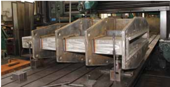
In-House Machining, 72" Bonneted Knife Gate Valve
