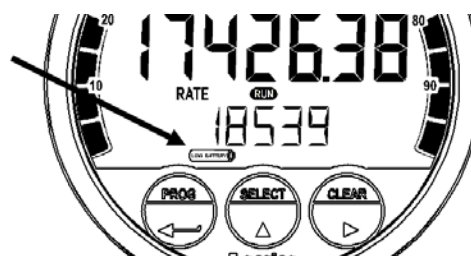
Fig. 7: Example of low-battery alarm
