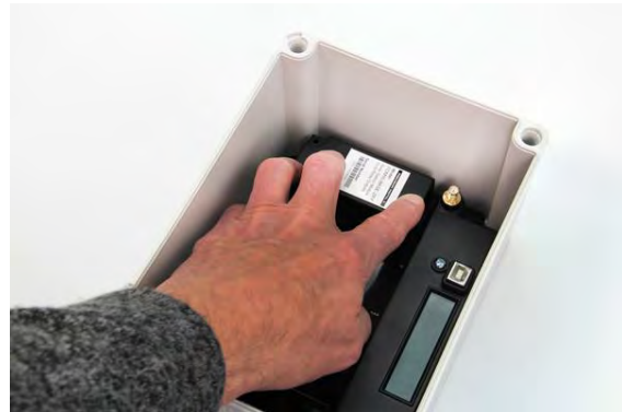
Press the module firmly into place to secure.
