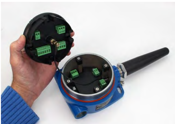
Relays Option Module Mounted on the Bottom of Enclosure (Install the module using the four screws provided)
