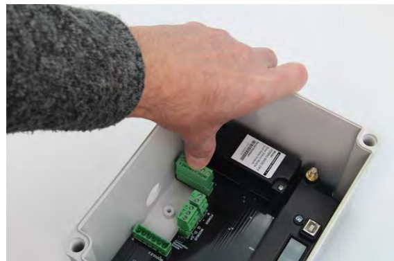
Press the connector plug firmly into place to secure.
