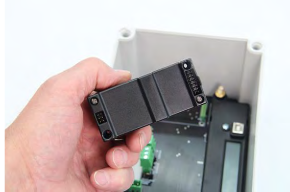
The back of the module contains the connector pins that plug into the connector board.
