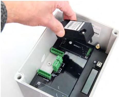
Insert the tab on the module into the slot on the connector board to line up and easily snap it into place.
