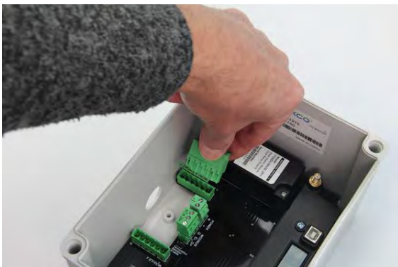
Connector plugs easily snap into the connector board.
