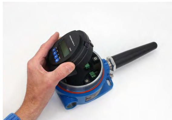
Display Module Mounted on Built-In Rails (Snap the module into place lining it up with the rail caps)
