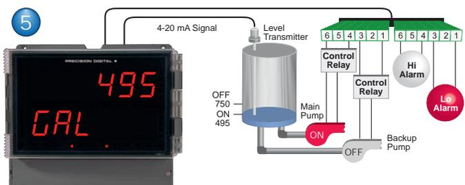
Relay #1 trips the Low Level Alarm at 495 gallons and resets at 750 gallons.
