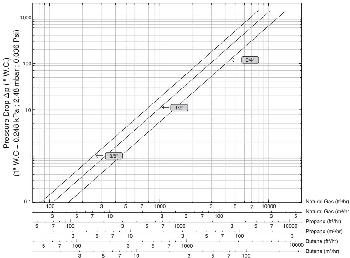
Note: Flow curves are based on the following standard conditions: 5 psi (0.3 bar) inlet pressure and 68°F (20°C) fluid temperature.
