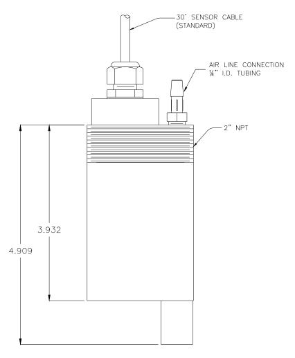
Figure 8 - Submersible S.O. Sensor Assembly
