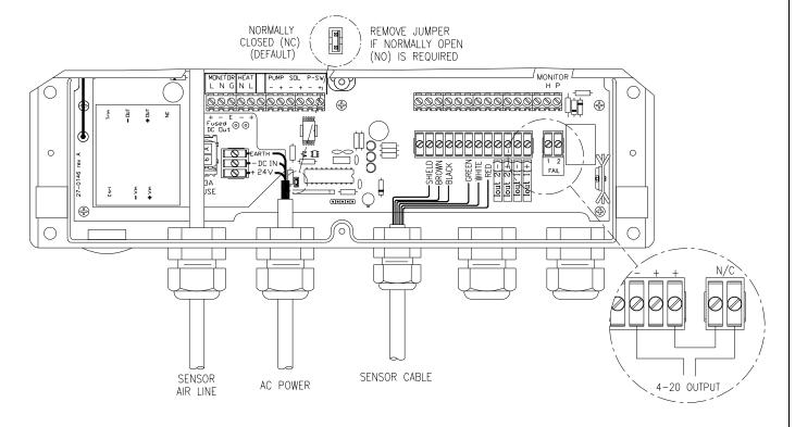
Figure 14 - Cleaner Failure & Jumper Map Config
