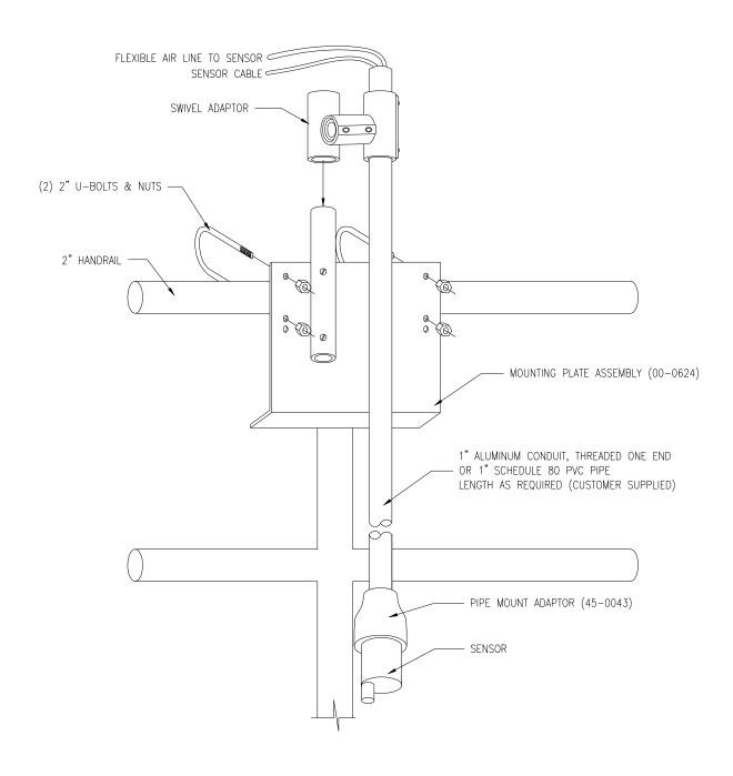
Figure 5 - Mounting Assembly Detail
