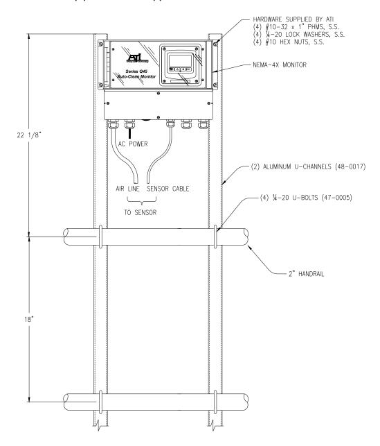
Figure 3 - Handrail Mounting Assembly
