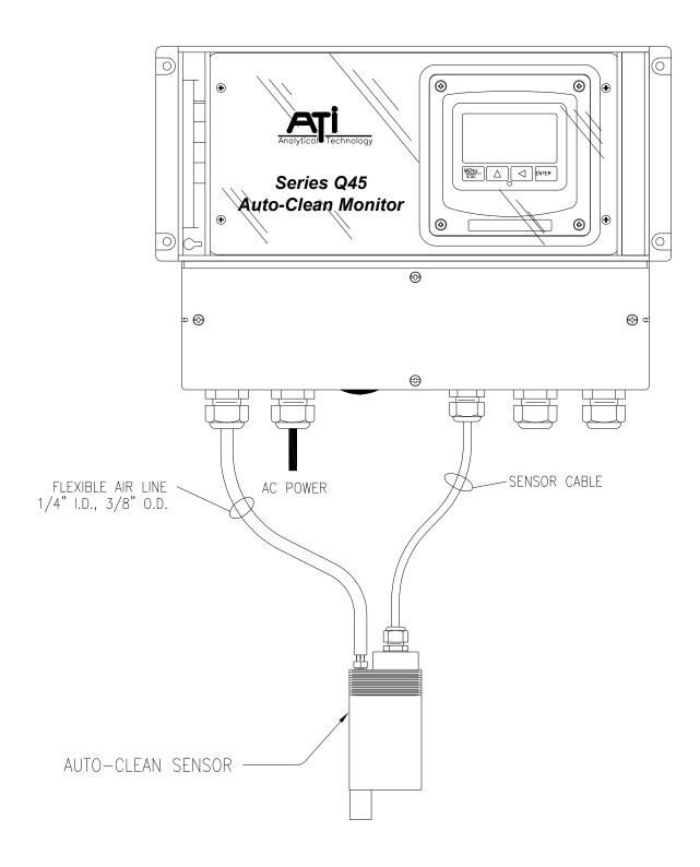
Figure 1 - D.O. System w/Auto-Clean Sensor
