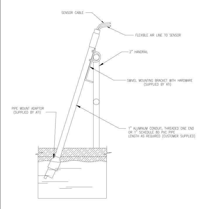
Figure 4 - Submersible Sensor Mounting Assembly
