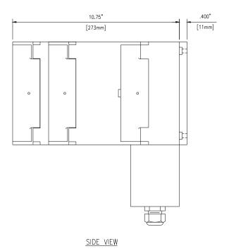
Figure 2 - Monitor Assembly Wall Mount Dim.
