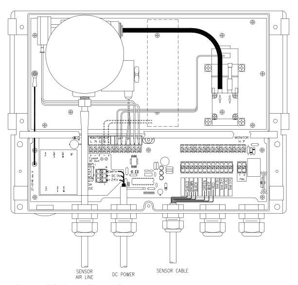
Figure 6 - D.O. Monitor Electrical Connections
