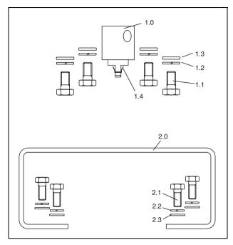
Fig. 11 Mounting kit for rotary actuators
