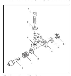
Fig. 6 Assembling the lever
