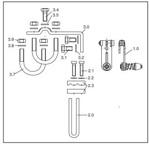
Fig. 4 Mounting kit for linear actuators
