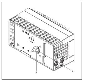
The arrow (1) on the feedback shaft (and thus the lever) must travel within the area marked with the small arrows (2).
