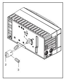
Fig. 12 Mounting the adapter
