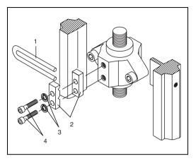
Fasten the follower guide (1) and the clamp plates (2) with screws (4) and spring washers (3) to the spindle of the actuator; hand-tighten the screws.
