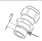
Apply the glue (Loctite 242 or similar) to the two last thread windings, approximately 7 mm from the end of the thread (see gray arrow in the illustration).
