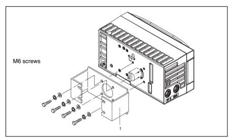
Fig. 13 Attaching the mounting bracket to the positioner
