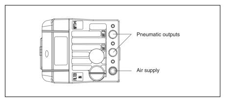
Fig. 15 Pneumatic connections
