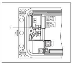
Fig. 22 Slide switch (service switch) of the shutdown module
