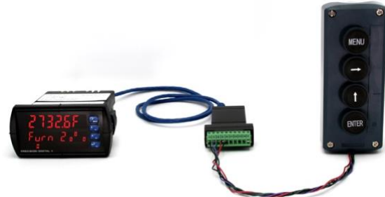
Figure 25. Meter to Control Station Connection
