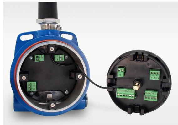
Display Module Connected to Antenna (Connect the antenna to the display module using the included antenna coupler)
