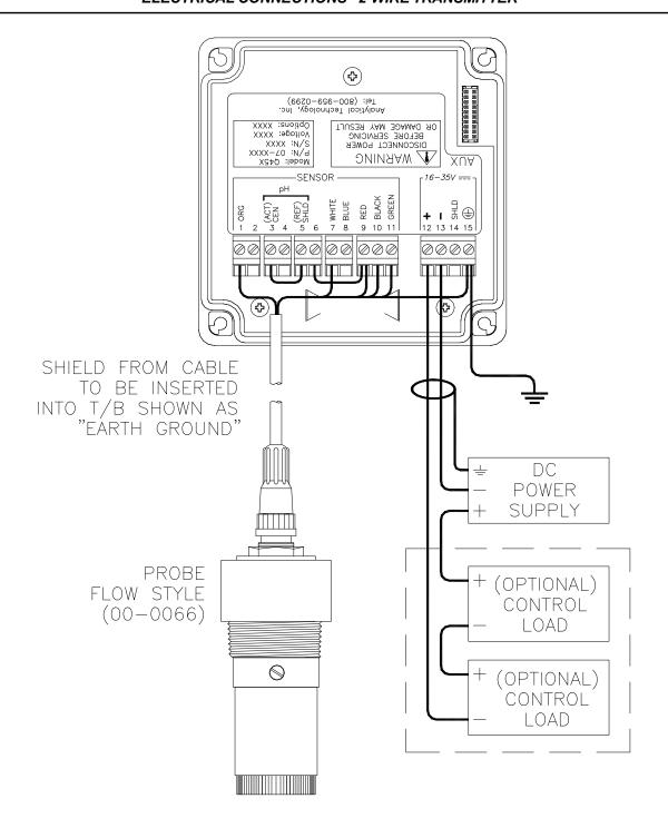
NOTES: 1. Voltage between Terminals 12 & 13 MUST be between 16 & 35 VDC.
