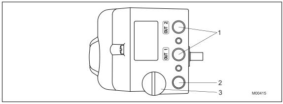
Fig. 18: Pneumatic connections
