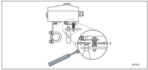
Fig. 8: Linkage for positioner
