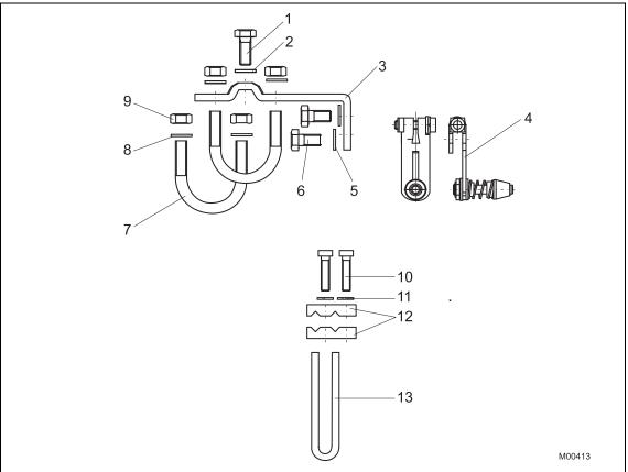
Fig. 3: Mounting kit for linear actuators
