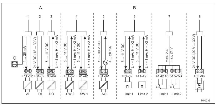
Fig. 13: Terminal connection diagram
