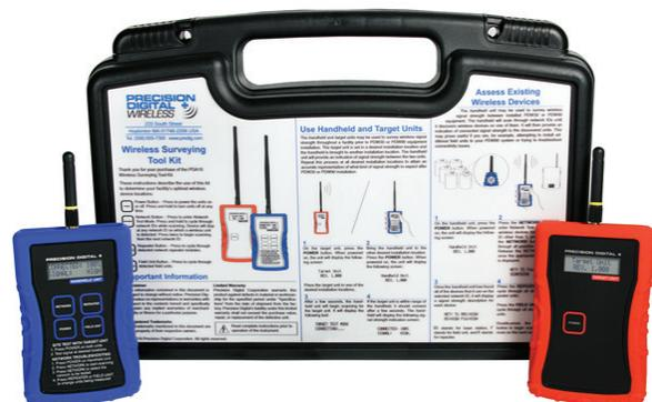
The handheld and target units are used to survey wireless signal strength throughout nonhazardous areas of a facility prior to PDW30 or PDW90 equipment installation. The target unit is set in a desired installation location and the handheld is brought to another installation location. The handheld unit will provide an indication of signal strength between the two units.
