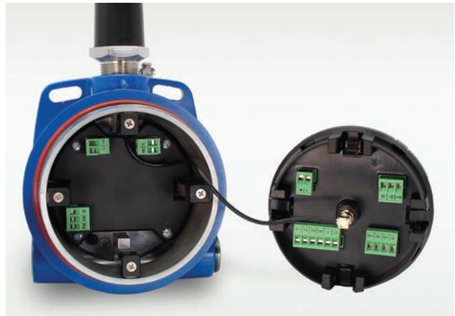
Display Module Connected to Antenna
