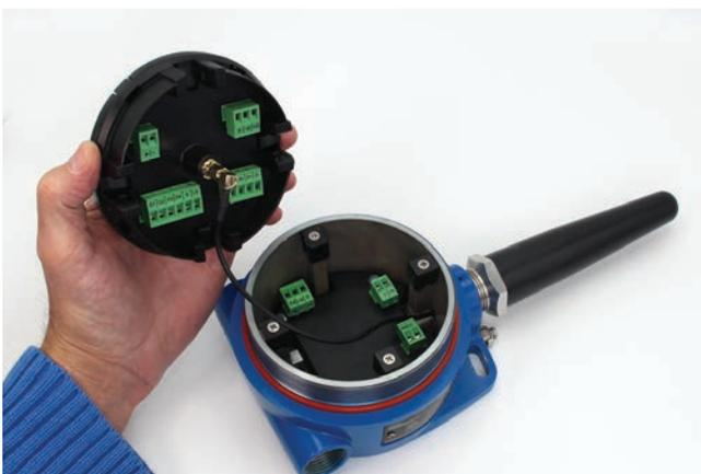
Relays Option Module Mounted on the Bottom of Enclosure
