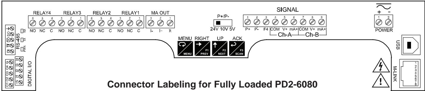
Connector Labeling for Fully Loaded PD2-6080
