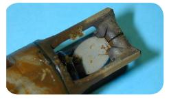
A reflector after accelerated testing of extremely harsh water, including rust, shows a virtually clean stainless steel reflector.
