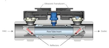
Cross-sectional view of meter showing location of flow tube, transducers and signal reflectors
