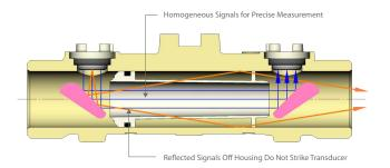
The electronic circuitry triggers the transducers, which generate and receive ultrasonic signals. In addition, the circuitry provides highly accurate time measurements through the use of complex pulse detection algorithms and digital signal processing.
