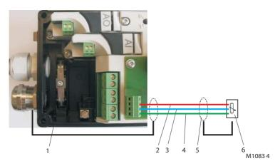
Fig. 29: Electrical connection
