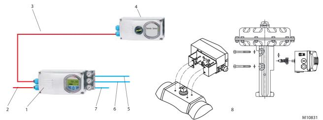
Fig. 26:D500 control unit made of stainless steel with D500 remote sensor made of stainless steel1Housing 1 (control unit) | 2 Setpoint | 3 Connection cable | 4 Housing 2 (remote sensor) | 5 Pneumatic output 2 |6Pneumatic output 1 | 7 Supply air | 8 Pneumatic drive
