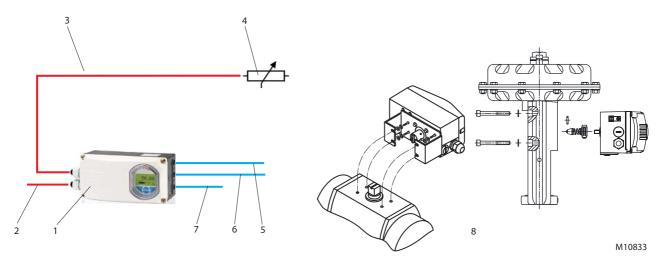
Fig. 28: D500 control unit for remote sensor
