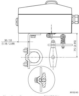
Fig. 23: Mounting to linear actuators to DIN/IEC 534
