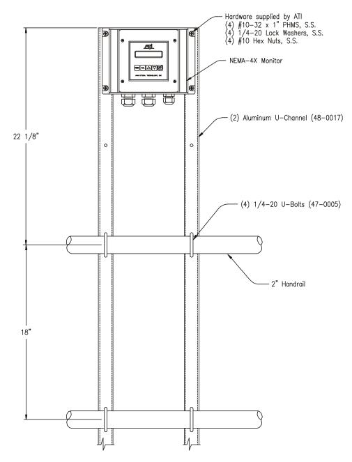
Figure 4 - Handrail Mounting Assembly
