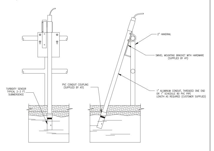
Figure 10 - Submersible Sensor Mounting
