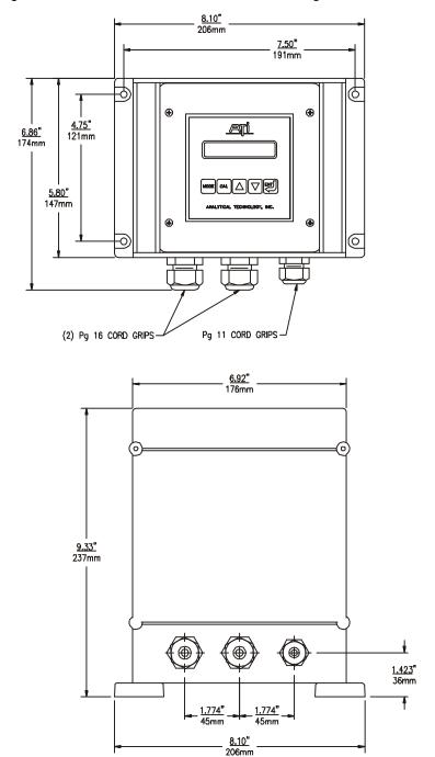
Figure 3 - Wall Mount Dimensions & Installation
