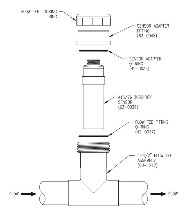
Figure 9 - Flow "T" Assembly
