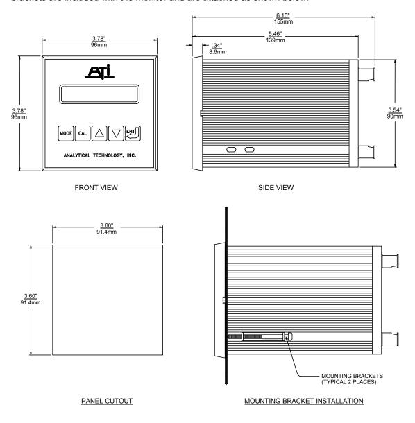
Figure 2 - Panel Mount Monitor Dimensions & Installation
