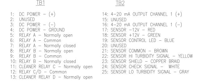
Figure 12 - DC Power / Sensor Connection Terminals
