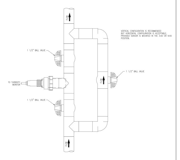
Figure 8 - Flow "T" Typical Configuration
