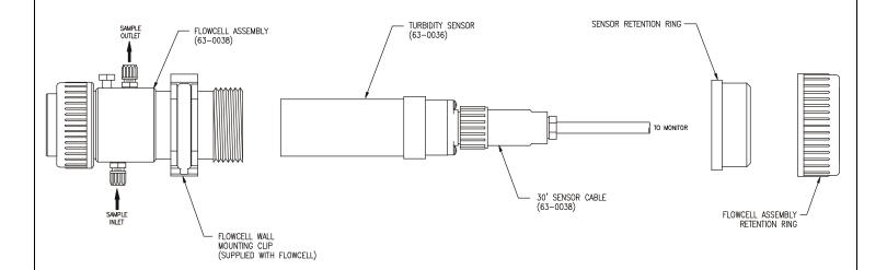
Figure 6 - Exploded Flowcell & Sensor Assembly
