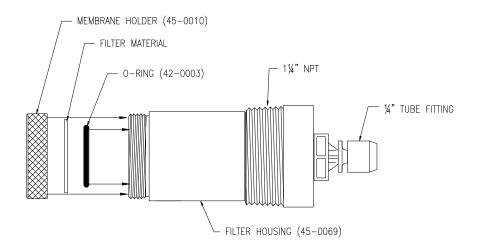
Figure 5 - Inlet Filter Assembly (ATI-0231)
