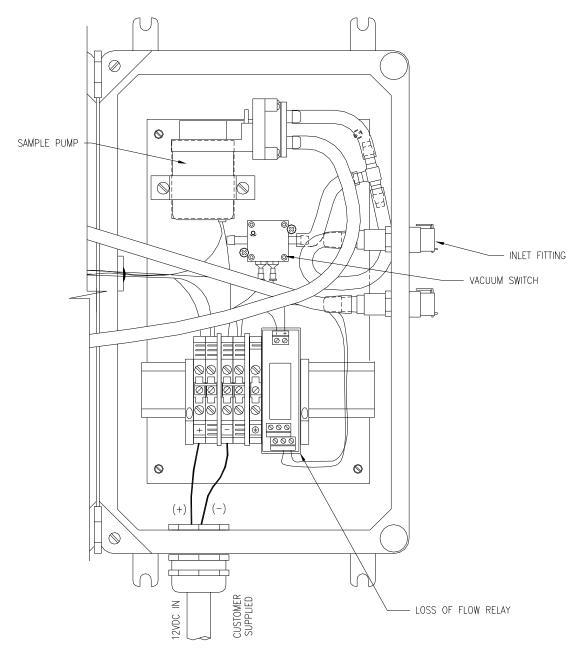
Figure 4 - Power and alarm output connections 12 VDC version (ATI-0331)
