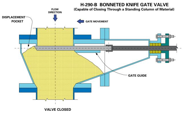
(Material is Pushed Into Displacement Pocket, Allowing the Valve to Close Fully)
