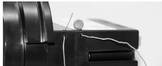
Figure 5: Wire Loop through Second Case Pass-Through
