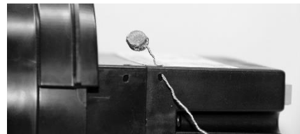
Figure 4: Wire Loop through Rear Case Pass-Through
