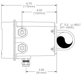
Figure 7 - Pipe Mounting Diagram
