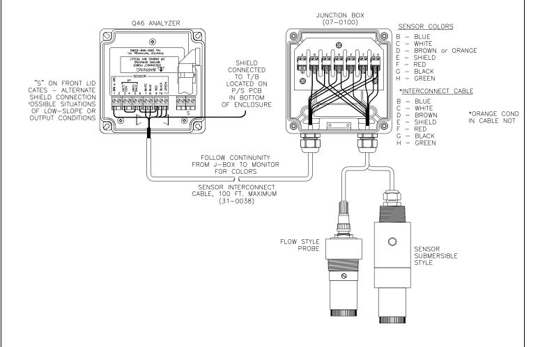
Figure 19 - Junction Box Interconnect Wiring
