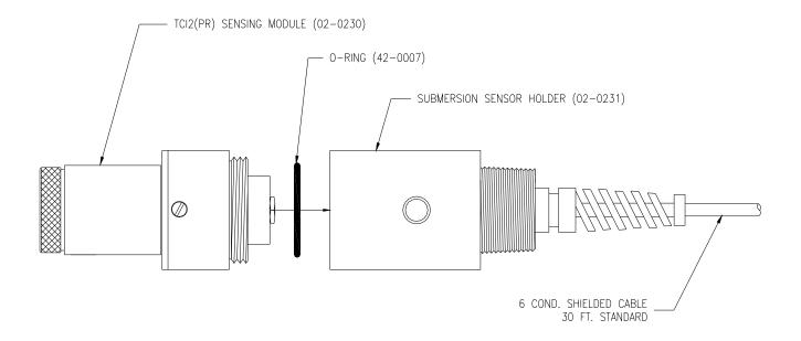
Figure 21 - Submersible Style Sensor Assembly
