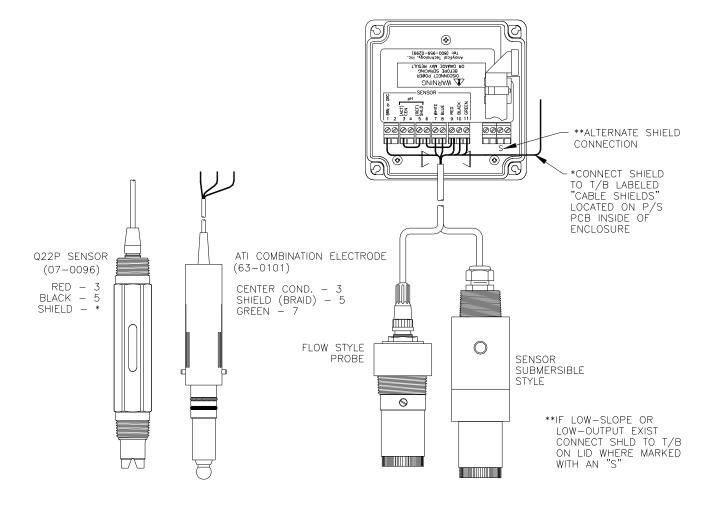
Figure 18 - Direct Sensor Connection
