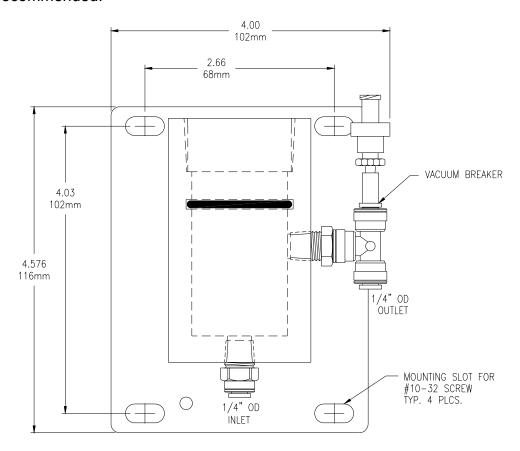
Figure 10 - Sealed Chlorine Flowcell Dimensions
