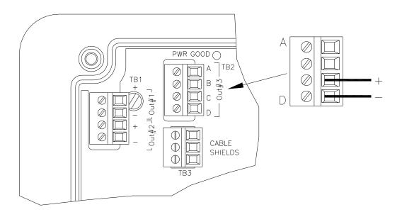
Figure 16 - Optional Analog Output Wiring
