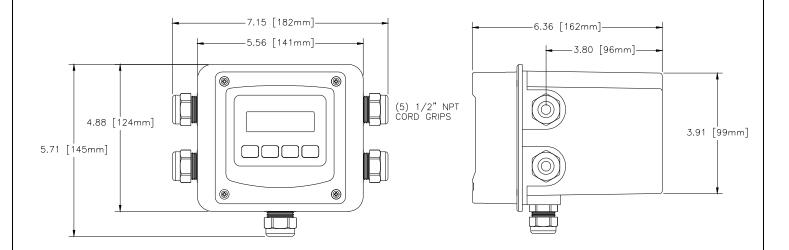
Figure 4 - Q46 Enclosure Dimensions
