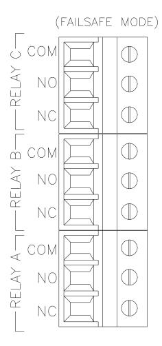
Figure 14 - Optional Relay Board Wiring
