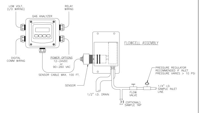
Figure 1 - Typical Monitoring System
