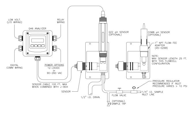
Figure 2 - Chlorine System w/Optional pH Bayonet Style Sensor
