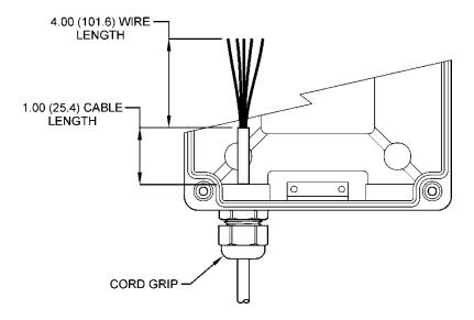
Figure 17 - Sensor Cable Preparation
