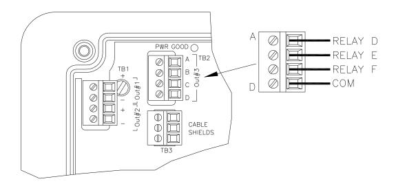
Figure 15 - Optional Relay Board Wiring
