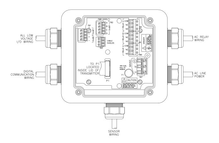
Figure 13 - Line Power Connection
