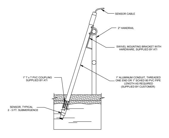
Figure 12 - Submersible Sensor Mounting
