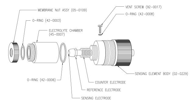
Figure 20 - Flow Style Sensor Assembly
