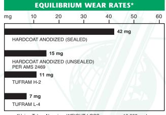
\*Using Taber Abrasion, WEIGHT LOSS = mg. per 10,000 cycles CS-17 wheel, 1000 gm. load
