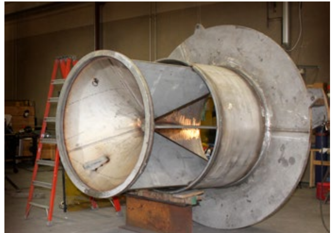
60" Fixed Cone Valve Body, Fabricated from 304 Stainless Steel & Nitronic 60
