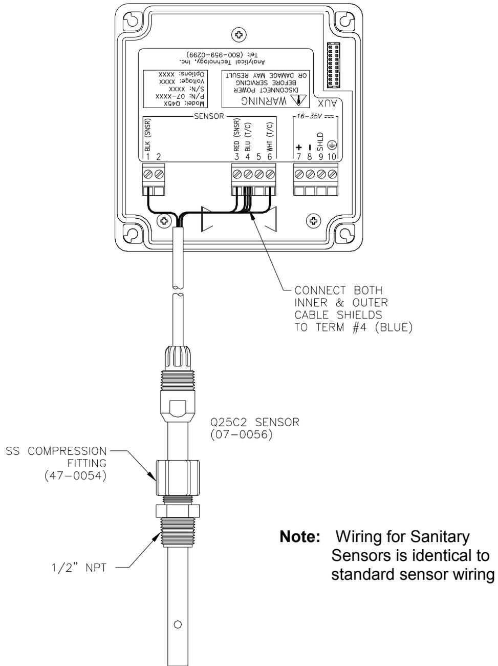
**Figure 3 - Sensor Connections**
