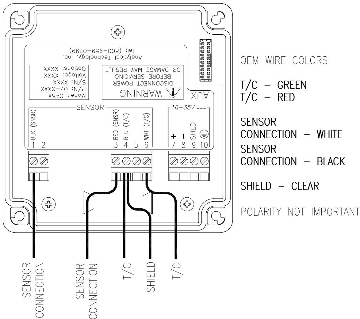
**Figure 4 - OEM Sensor Connections**
