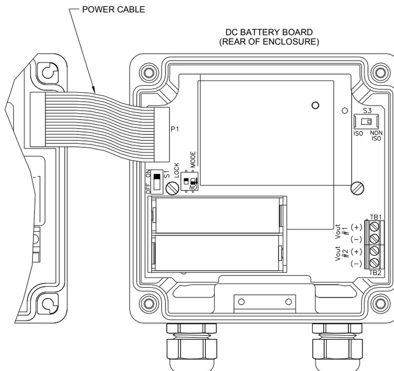
**Figure 5 - Battery Board Connections**
