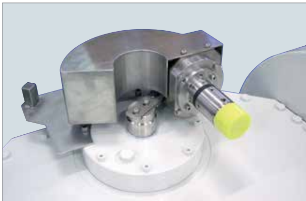
Position transducer assembly with electrical instrumentation connector.
