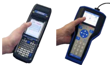
Figure 1. Left: ECOM, Right: Rosemount 475. The CVA can be configured using a Bluetooth wireless enabled device such as a PC or alternatively a typical shop HART communicator such as an ECOM or Rosemount 475
