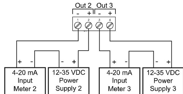
Figure 4. Dual Analog Output Module Connections
