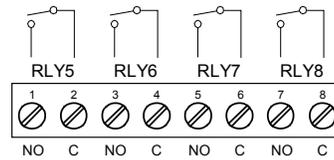
Figure 3. External Relays Module Connections
