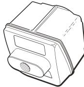
HM2-RT1 and RT2 modules are RTD temperature measurement modules compatible with Pt100, Pt1000, Ni120, Cu10, and up to six user programmable resistance curves. Measurements can be displayed in degrees Fahrenheit, Celsius, Kelvin, Rankin or ohms. The setup menu allows the operator to choose configurations for 2, 3 or 4 wire RTD probes. In addition, the setup menu also allows selection of 1, 0.1, 0.01 or 0.001 decimals of resolution. Accuracy specifications are detailed in the data sheet.
