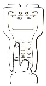
When powering on, the LCD display will briefly indicate the calibrator model number, serial number, owner information and whether it is an intrinsically safe or not intrinsically safe model. If pressure or temperature modules are installed, serial
