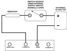
\*Resistor should be sized to allow current as follows: 2 mA < I < 36 mA, 2 mA  $\approx$  12 k  $\Omega$ , 35 mA  $\approx$  686  $\Omega$
