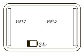
If the power supply has been overloaded and a warning message shows on the display (supply current is specified at 35ma and will overload at approximately 54-55ma)
