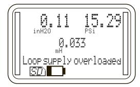
Remove the overload from test circuit and enable the 24 VDC power supply via MENU commands. (See section 14k)
