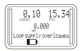
Remove the excessive load from the circuit and attempt to activate the 24v loop power supply via the MENU as described above.
