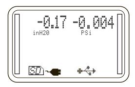
The HHC is now ready for basic pressure or temperature measurement.
