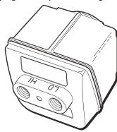
HM2-2 are high pressure measurement devices. They are single-port modules based on sensors capable of measuring gauge, absolute, compound or vacuum with ranges spanning from vacuum to 5 psi to 10,000 psi. All wetted parts are 316 stainless steel (except for 10k psi module which has 17-4ph stainless steel) and are intended for use with any pressure medium compatible with stainless steel.
