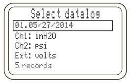
Use up and DOWN ARROWs to scroll through saved Datalogs. Press ENTER when desired name appears Review Data screen appears
