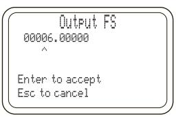
Press left and RIGHT ARROWs to position cursor beneath desired numeric character
