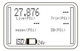
In Switch Test Mode the display will initially show the Live pressure (pressure being applied at that time), and units of measure. The switch trip point, reset point and dead band (DB) will be blank indicated by "---"
