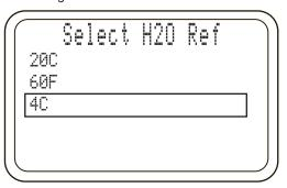
Press ENTER to select temperature and exit to Measurement Mode.
