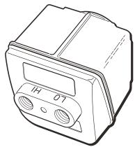
Note: When making connections to pressure ports on Quick-Select modules always use proper tools such as the proper size wrench, slip joint pliers or locking jaw pliers to hold the stainless steel manifold and use a second tool such as a properly sized wrench to tighten the connection. NEVER tighten the fitting by holding it only in the base unit
