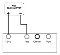
4/20 TRANSMITTER HOOK UP USING, EXTERNAL SUPPLY
