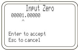
Press left and RIGHT ARROWs to position cursor (^) beneath desired numeric character.
