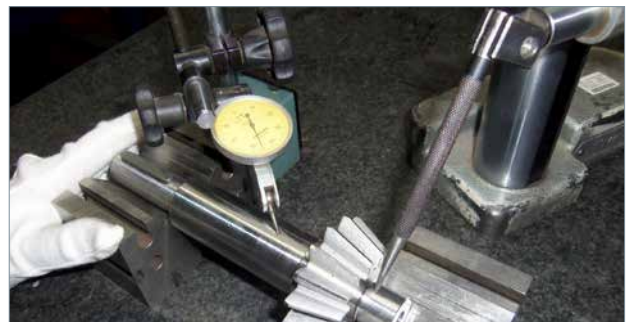
Concentricity test with dial indicator.
