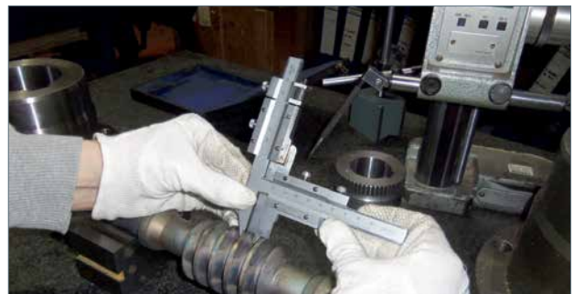
Gear teeth dimension check with vernier gear tooth.
