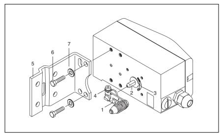
Fig. 7 Mounting lever and angle bracket to TZIDC-110
