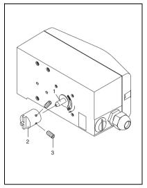
Fig. 12 Mounting the adapter
