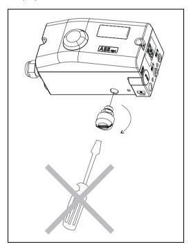
Fig. 16 Mounting the splash guard cap
