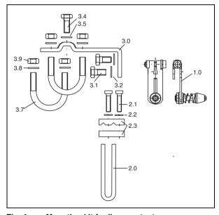
Fig. 4 Mounting kit for linear actuators
