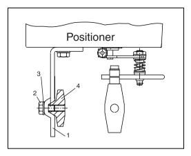
Fasten the angle bracket (1) with screw (2), plain washer (3) to the cast iron yoke (4).
