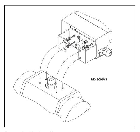
Fig. 14 Attaching the positioner to the actuator
