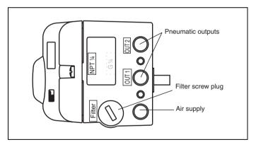
Fig. 15 Pneumatic connections
