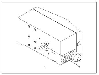
The arrow (1) on the feedback shaft (and thus the lever) must travel within the area marked with the small arrows (2).
