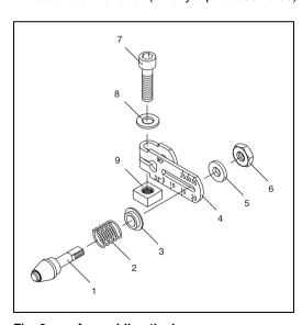
Fig. 6 Assembling the lever
