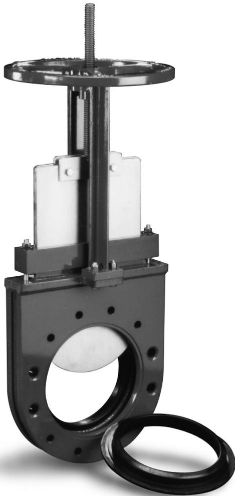
The Red Valve Series D Flexgate Slurry Knife Gate Valve is a 100% full bore, truly bi-directional valve designed for tough slurry applications. The Flexgate features heavy-duty elastomer seat cartridges which provide droptight closure and are replaced **WITHOUT ANY VALVE DISASSEMBLY**, for ease of maintenance.
