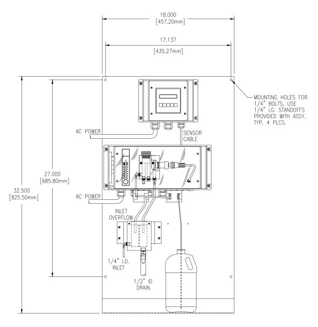
Figure 1 - Typical Res. SO2 Monitoring System
