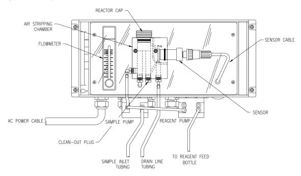
Figure 7 - Chemistry Module Layout
