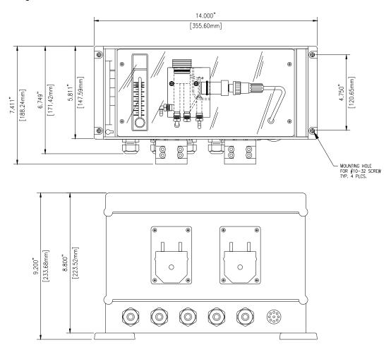
Figure 4 - Chemistry Module Dimensions
