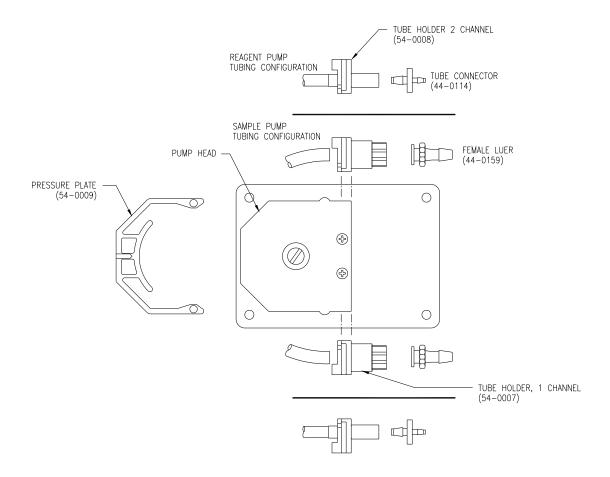
Figure 11 - Pump Head Assembly Exploded View
