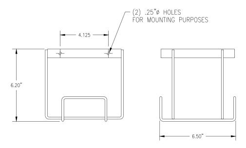
Figure 8 - Reagent Bottle Mounting Bracket
