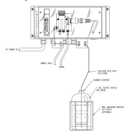
Figure 9 - Solution Feed Assembly
