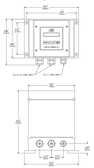
Figure 3 - Nexa 4X Wall Mount Dim. & Installation
