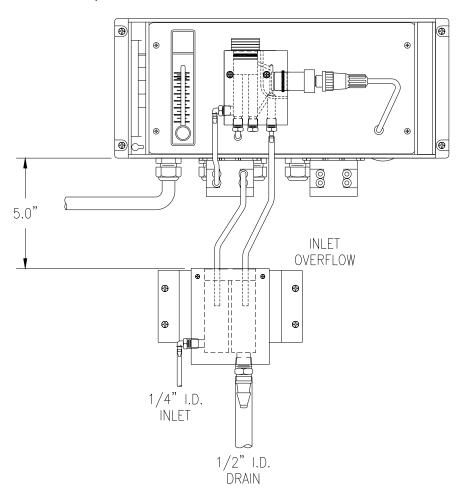
Figure 10 - Sample Inlet Overflow Arrangement
