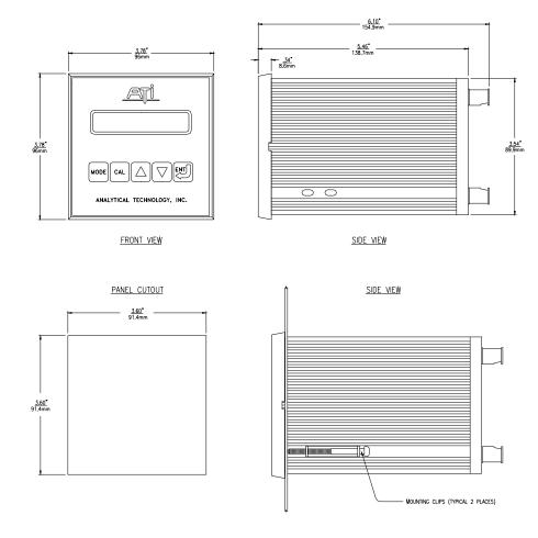
Figure 2 - Panel Mount Dim. & Installation
