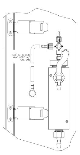
Figure 16 - Inlet Filter Block Assembly
