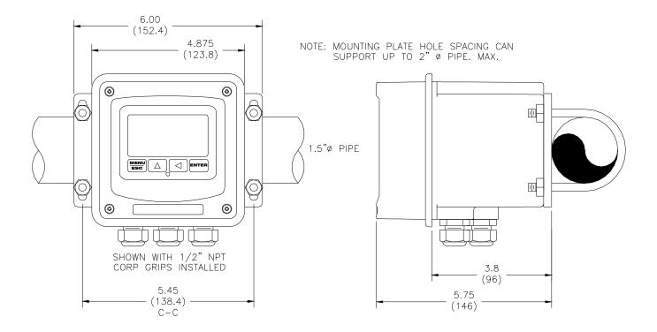
Figure 6 - Pipe Mounting Diagram
