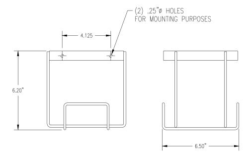
Figure 15 - Reagent Bottle Holder Dimensions
