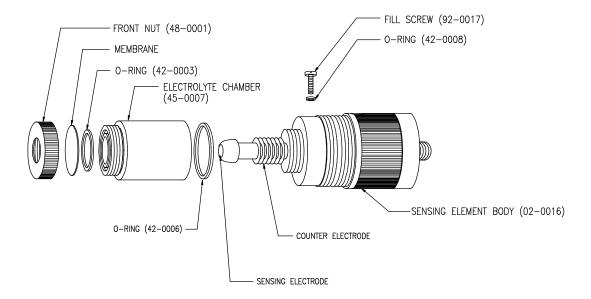
Figure 13 - Sensor Assembly
