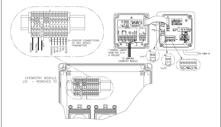
Figure 12 - Electrical Connections - Separated System
