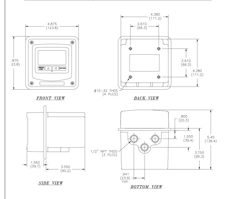
Figure 3 - Q45 Enclosure Dimensions
