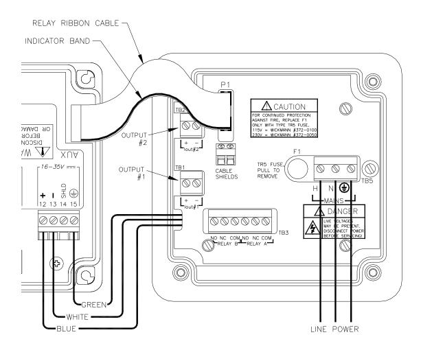
Figure 9 - Line Power Connection
