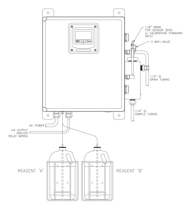
Figure 1 - Q45N with Integral Monitor & Chemistry Units
