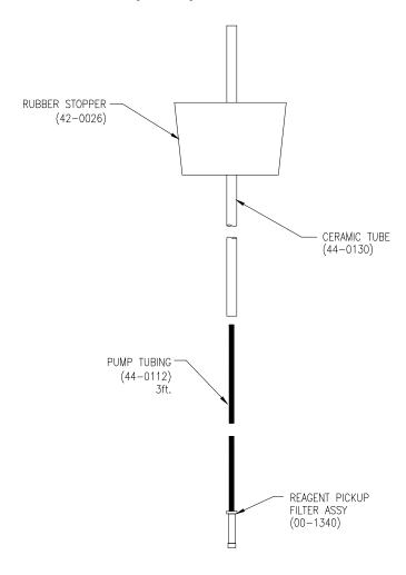
Figure 14 - Reagent Pickup Assembly
