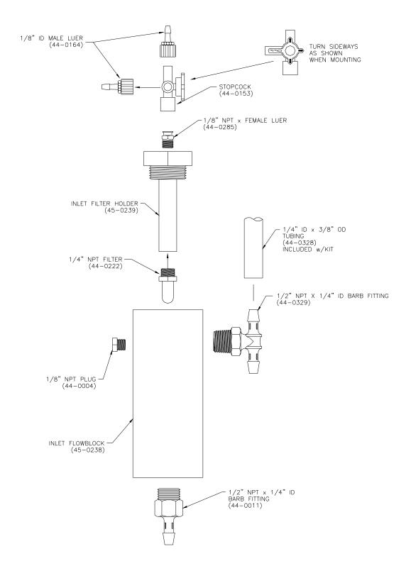
Figure 22 - Inlet Flow block Exploded View
