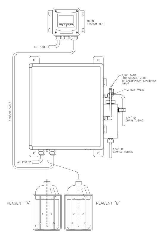
Figure 2 - Q45N with Separate Monitor & Chemistry Units
