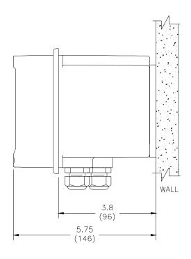
Figure 5 - Wall Mounting Diagram
