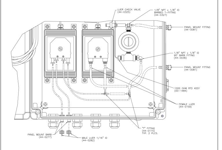
Figure 23 - System Fittings Exploded View
