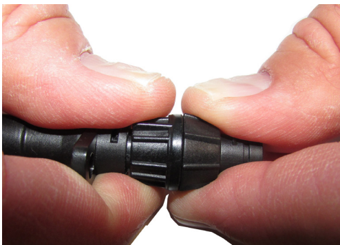
Figure 1: Twist the collar on the connector
