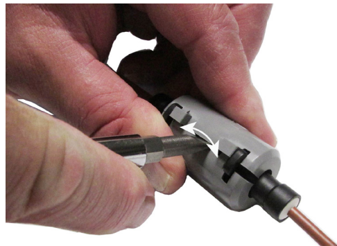
Figure 6: Removing the security cover
