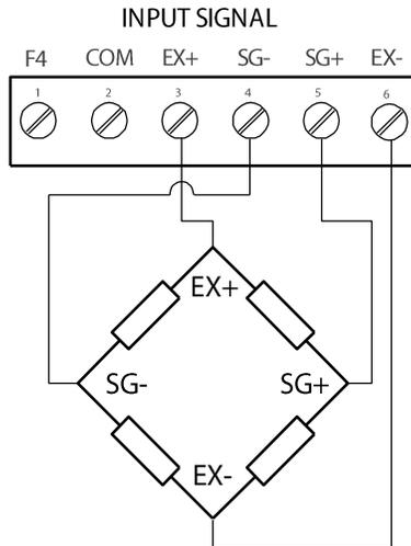
**Figure 10. Strain Gauge Powered by Internal Supply**
