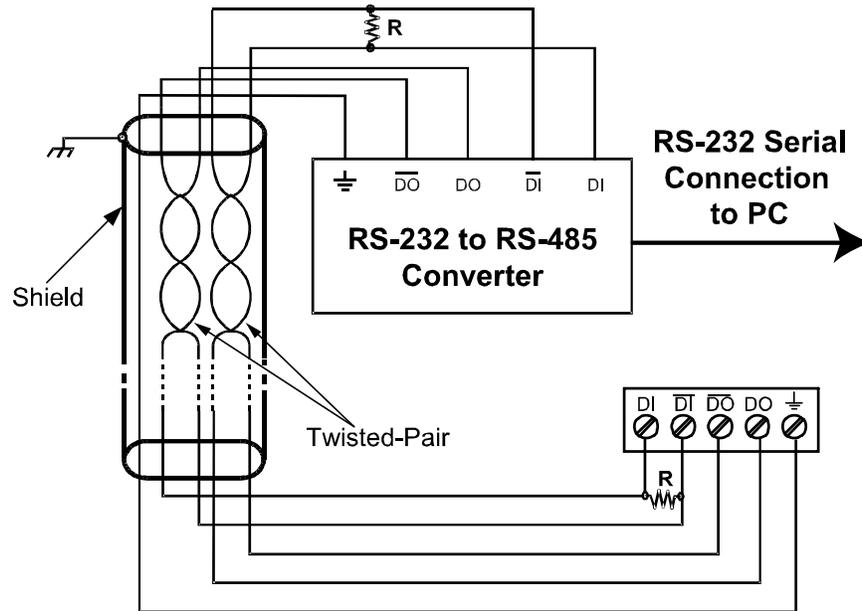
Figure 18. RS-422 or RS-485 Wiring
