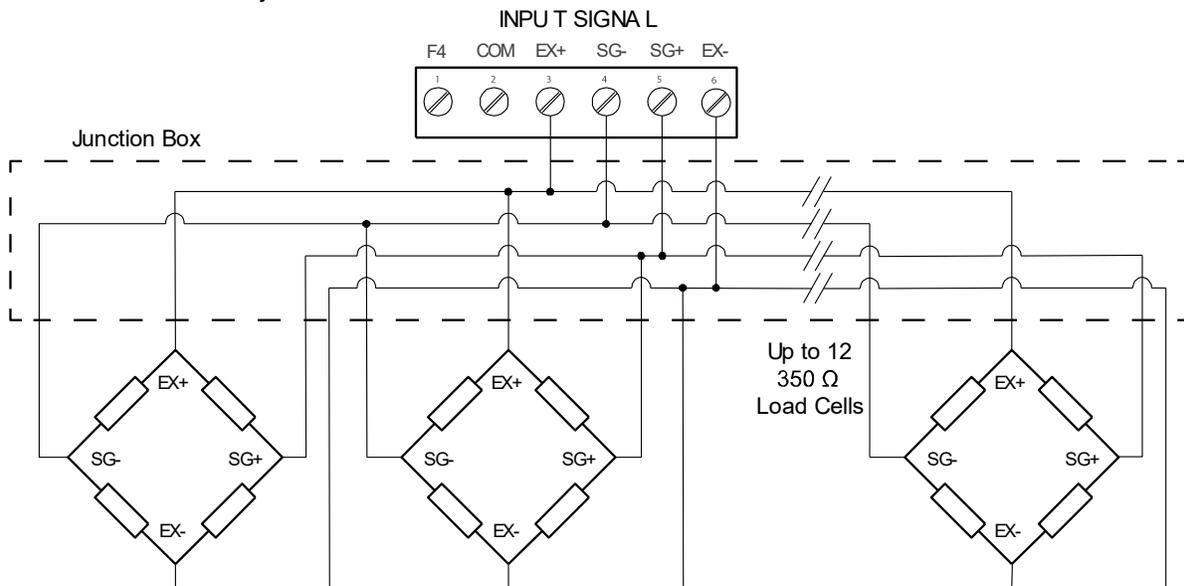
**Figure 12. Multiple Strain Gauges Connected Through Junction Box**
