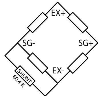
**Figure 14. Shunt Resistor**
