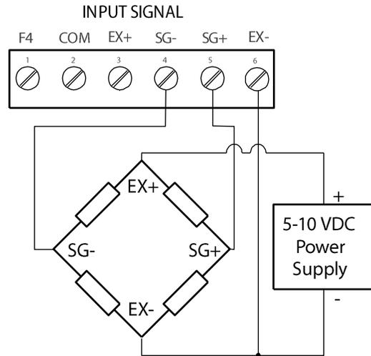
**Figure 11. Strain Gauge Powered by External Supply**
