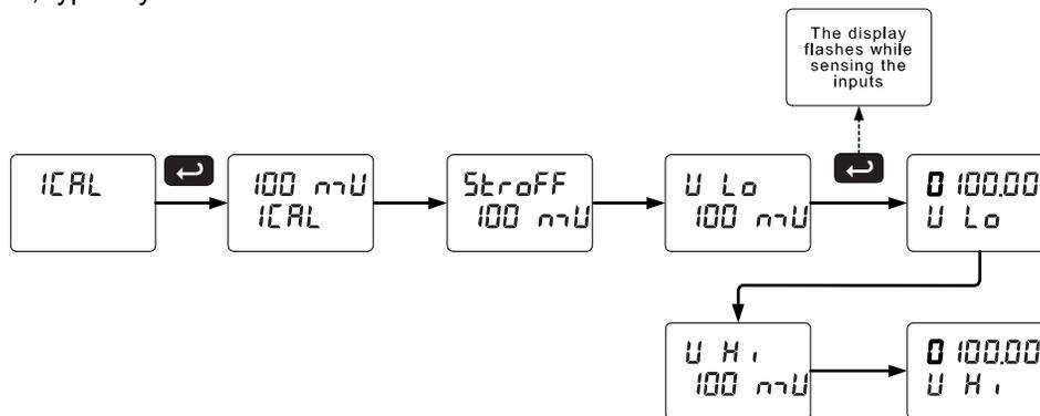
The graphic above shows the calibration of the 100 mV input range. The other input ranges are calibrated in a similar way.
