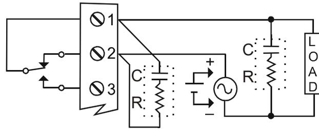
**Figure 16. AC and DC Loads Protection**
