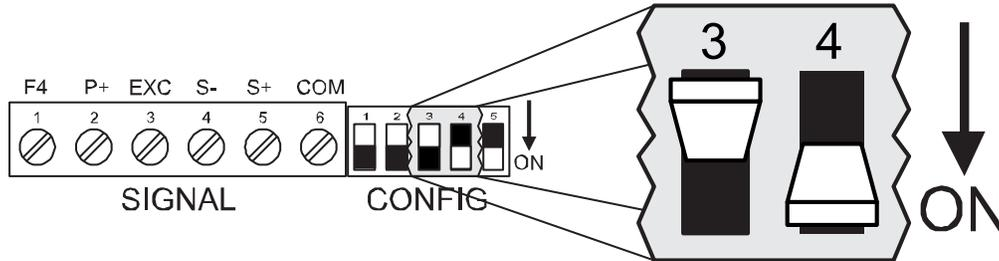
**Figure 9. Strain Gauge Configuration Switch**
