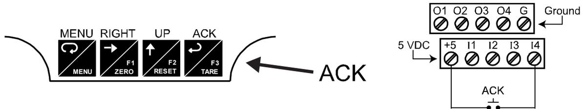
**Figure 26. Acknowledge Relays w/Function Key or Digital Input**
