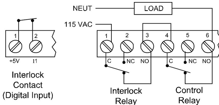
Figure 25. Interlock Connections
