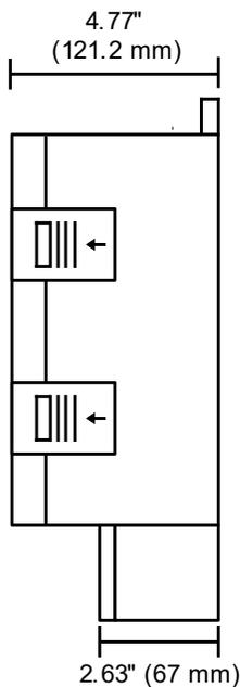
Figure 2. Meter Dimensions - Side View
