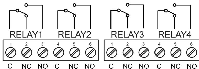
**Figure 15. Relay Connections**
