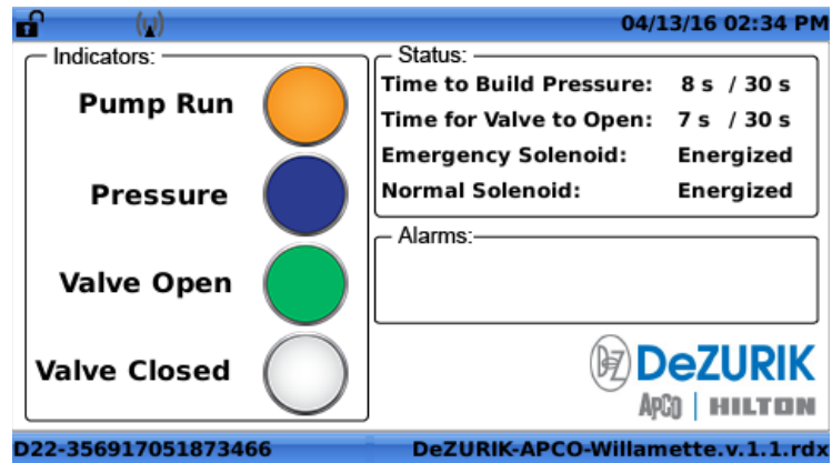
Figure 17A. ECB-CP Controller Home Screen, Normal Operation
