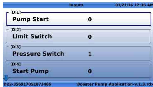
Figure 22: PC-22D Controller, input status.
