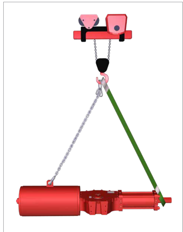
Fig 7.1 Lifting (single-acting actuator up to size 161)
