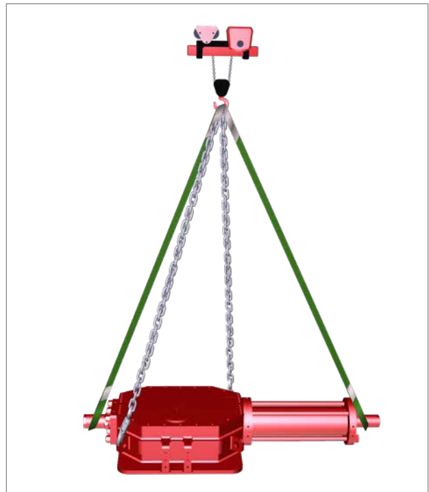
Fig 7.4 Lifting (double-acting actuator size 200 - 350)
