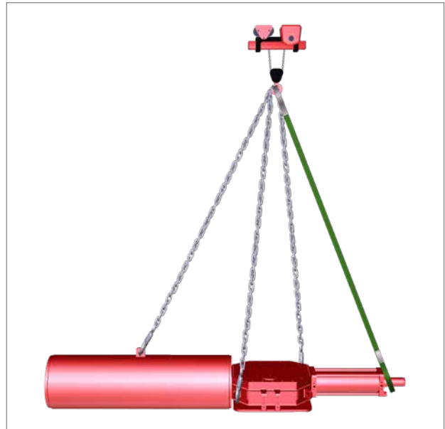
Fig 7.3 Lifting (single-acting actuator size 200 - 350)
