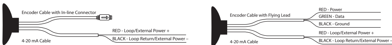
Figure 3: HR-E LCD 4-20 wiring options
