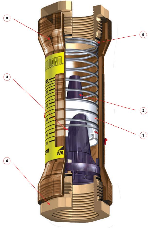
The flow meter is a variable area instrument. A sharp-edged orifice, located within the piston assembly, forms an annular opening with the contoured metering cone. The piston assembly carries a cylindrical PPS/ceramic magnet that is magnetically coupled to an external indicating magnet which moves precisely in direct response to movement of the piston. A calibrated spring opposes flow in the forward direction.
