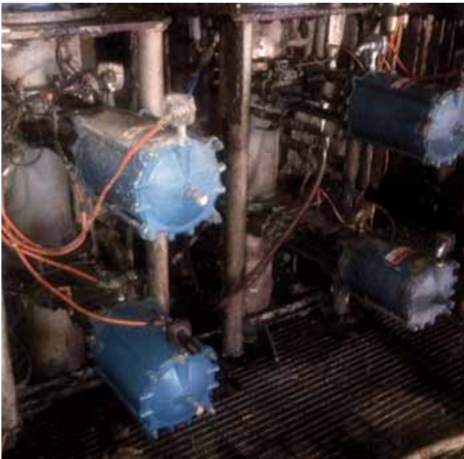
Metal seated KGC-MD Maximum Duty Knife Gate Valves installed in High Density (HD) cyclone separators at a recycle paper mill. These valves lasted three times longer than the previous valves installed in this service.
