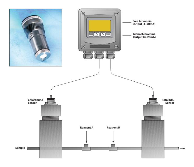
Chloramination is increasingly being used in potable water systems to limit THM formation and insure disinfection in large distribution systems. Proper control of this process requires the addition of sufficient ammonia to insure that only monochloramine is formed while limiting the amount of excess ammonia to a minimum.
