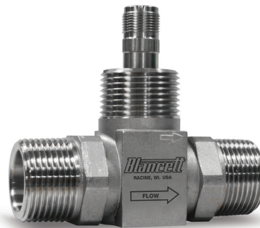
Figure 3. Blancett model 1100 turbine flow meter provides an accuracy of \pm 1\% of reading and operating temperatures of -150^{\circ}\text{F} \dots 350^{\circ}\text{F} ( -101^{\circ}\text{C} \dots 177^{\circ}\text{C} ).
