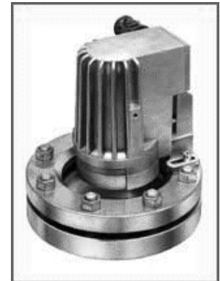
CHEMLUX sightglass light fitting type PEL 50 deHSch, EEx de IIC T4, 50 W, on VETROLUX sight-glass to DIN 28120
