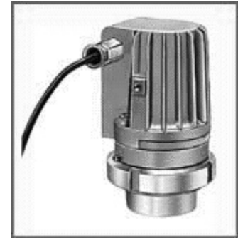
CHEMLUX sightglass light fitting type FKEL 20dHR, EEx d IIC T4, 20 W, on VETROLUX screwed sightglass similar to DIN 11851, DN 65
