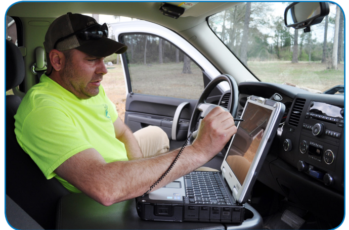
Meter Reader Mark Waldo collects a drive-by read using the utility's ORION Classic (CE) mobile reading system.
