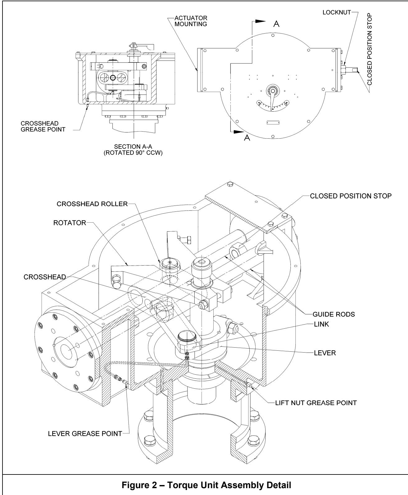
**Figure 2 – Torque Unit Assembly Detail**
