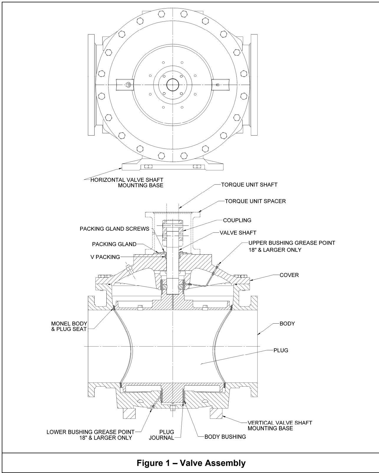
**Figure 1 – Valve Assembly**
