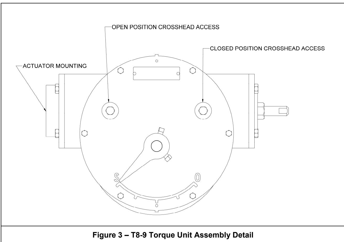
**Figure 3 – T8-9 Torque Unit Assembly Detail**
